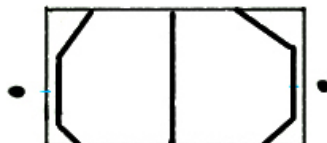
Zoomed In, Telephoto Vanishing points move apart as the scene grows larger, leaving the original perspective intact.
